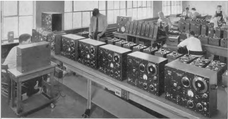
A portion of the standardizing laboratory at the General Radio Company. In the foreground are several TYPE 605-B Standard-Signal Generators undergoing calibration.
